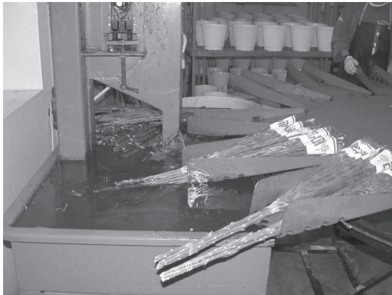
Figure 14 A commercial stem cutter that cuts stem ends while under water.
